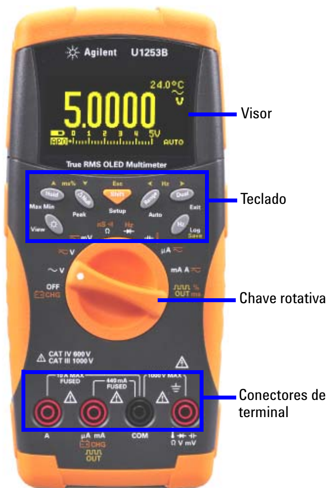
Figura 1-4 Painel frontal do U1253B
